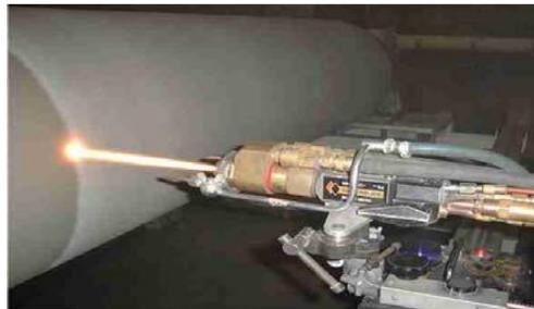
Figure 1. Detonation gun spray system set up
